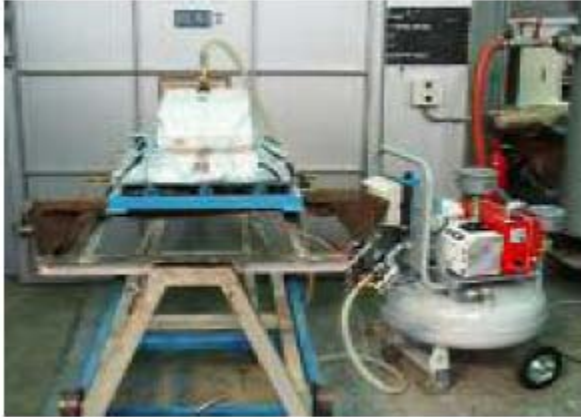
Fig. 21: Tool and vacuum pump system
