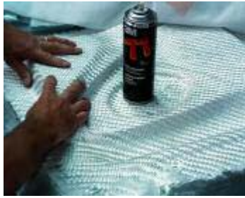
Fig. 14: Draping the Twintex®
