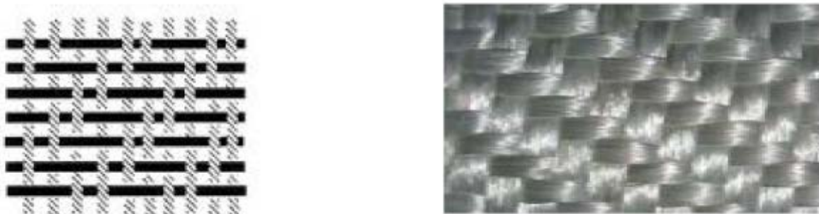
Fig. 12: Twill weave (Twintex® 1-1, 745 g/m 2 or 1485 g/m 2 , 60%)
