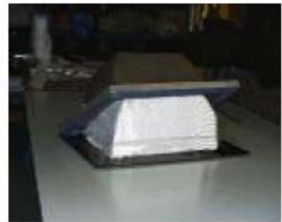
Fig. 20: Silicone membrane molding.
